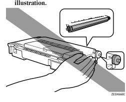
Set the development unit by aligning the guides, pushing towards direction ((1)), and then inserting slowly until it stops (2).
