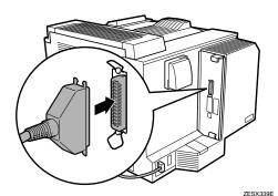
Attach the other end of the parallel cable to the port of the computer. Secure the cable.
