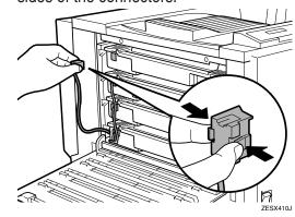
Follow steps 4 to 8 for each development unit individually. Remove the development unit by lifting it first as shown in the illustration (1) ⇒
