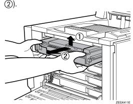
The illustration shows how to remove the black development unit. The procedure is the same for all four colors.
