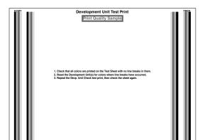
The development sheet that comes with the machine is a sample of correct print. If the test page's colors are blurred or broken compared to this sheet, turn the printer off, and then reset the development unit using the following procedure.
