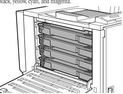
Remove all of the packing materials with red tags. Four packing materials are connected together, and there are two of them. Remove one by one from the top of the units by holding the packing material, not the wire.
