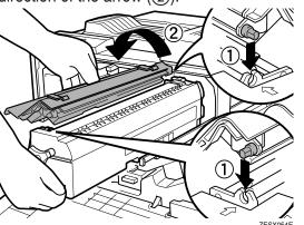
Remove the two red fittings along with the tapes from the fuser oil unit.
