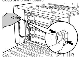
Pull out the development unit partially (approximately 30mm 1) by lifting it first as shown in the illustration.
