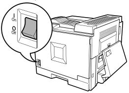
When the power is turned on, the following message appears on the panel display for approximately 15 minutes while the machine is being warmed up.
