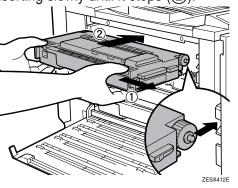
The illustration shows how to install the black development unit. The procedure is the same for all four colors.
