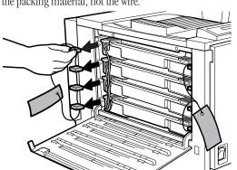
Detach the connectors from the development units from the top to the bottom by pressing the sides of the connectors.
