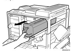
Take out the new fuser oil unit from the bag. Remove the covering paper, the seals, and then the fitting.
