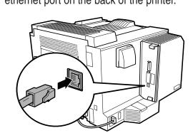
Connect the other end of the cable to the network such as hub.
