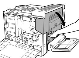
Remove the packing materials by holding the red
