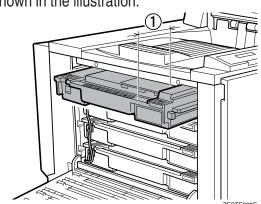
The illustration shows how to pull out the black development unit. The procedure is the same for all four colors.
