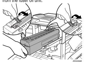
Holding the handle, insert the fusing unit slowly
